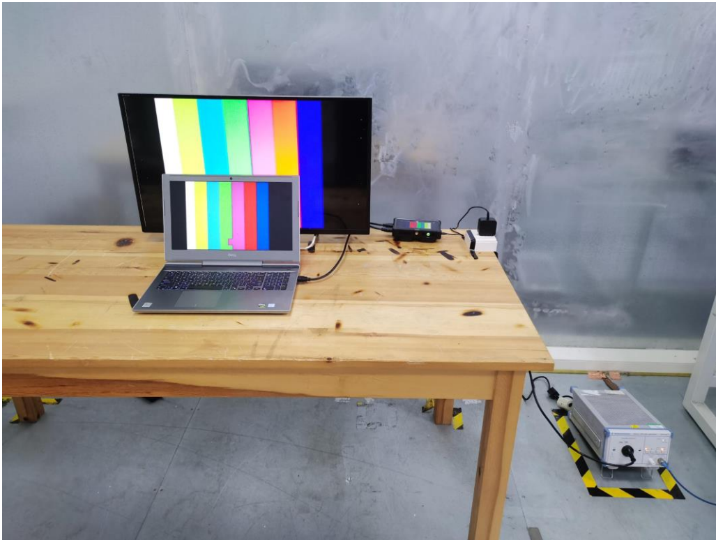
Photo of Power Line Conducted Measurement
