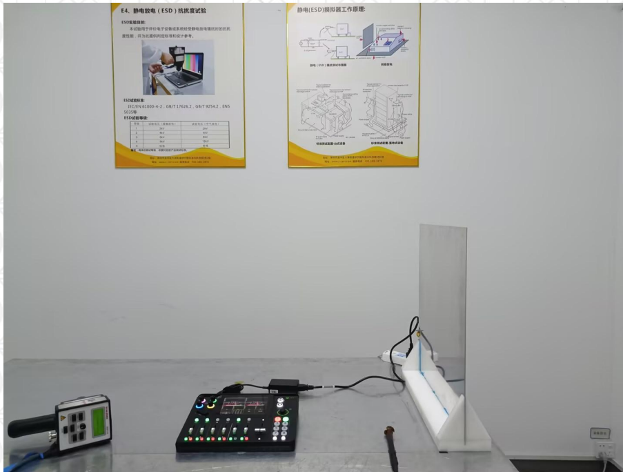
Figure 5: Electrostatic Discharge Test Setup
