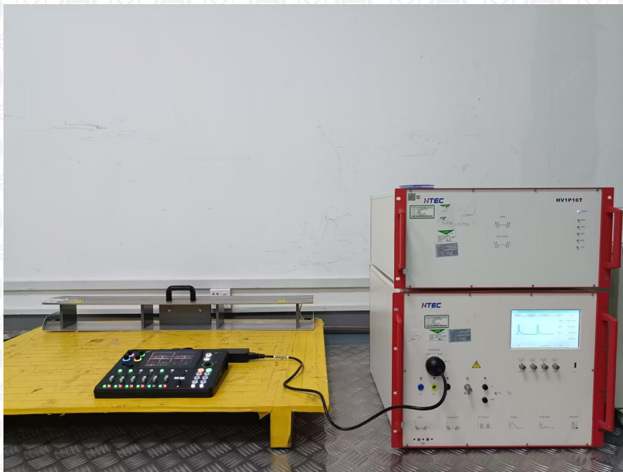
Figure 6: SURGE、DIP&EFT Test Setup
