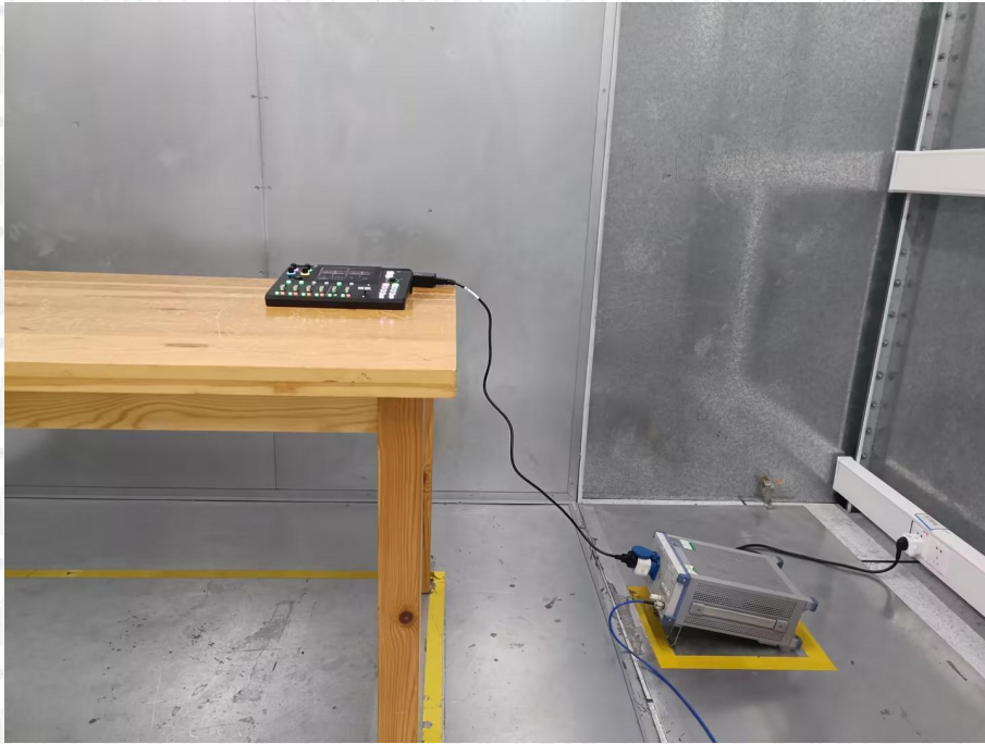
Figure 3: Conducted Emission Test Setup
